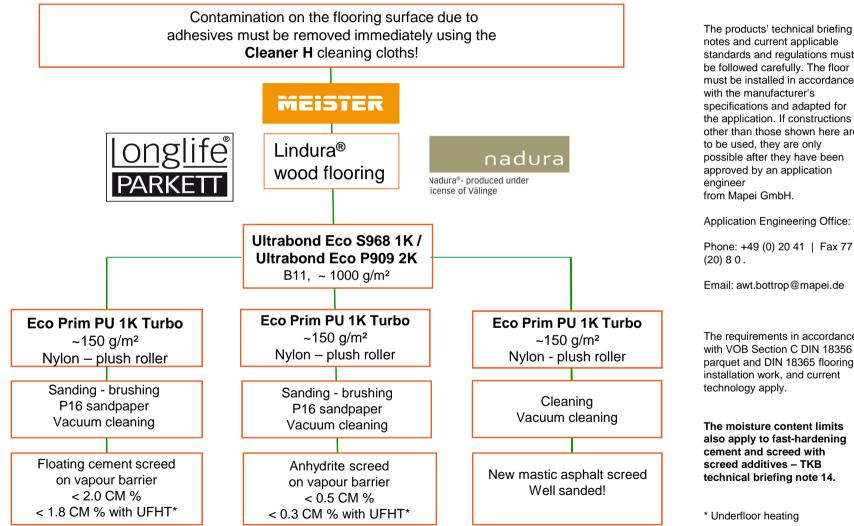
notes and current applicable standards and regulations must be followed carefully. The floor must be installed in accordance with the manufacturer's specifications and adapted for the application. If constructions other than those shown here are to be used, they are only possible after they have been approved by an application engineer from Mapei GmbH. Application Engineering Office:
